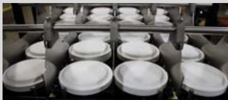
1 - MULTI-LANE ACCUMULATION Accumulates multiple lanes of product on single conveyor
