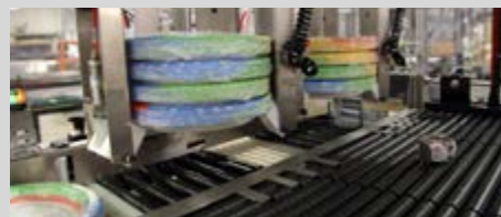
4 - PLATE BUNDLE STACKING Upstacking of product after wrapping for case packing
