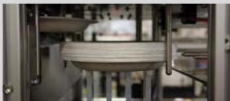
3 - SINGLE PLATE STACKING Lift grid gradually lowers as stack increases to allow for various stack heights
