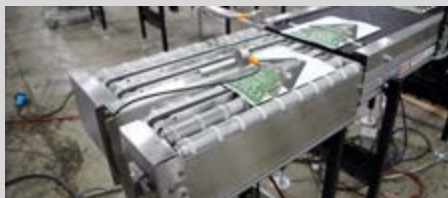
1 - HIGH-SPEED LIFT AND TRANSFER Accurate product transfer at 90-degree angle
