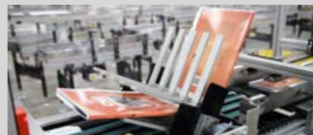
4 - FLIPPER Orients product based on process needs
