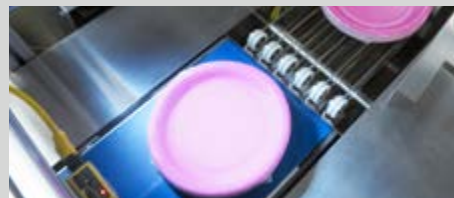
2 - REJECT DEVICE Ensures quality control for maintaining product integrity
