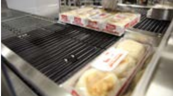
LANE COMBINING WITH AN OVERHEAD PUSHER
