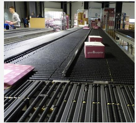
Shuttleworth's Slip-Torque® roller technology
