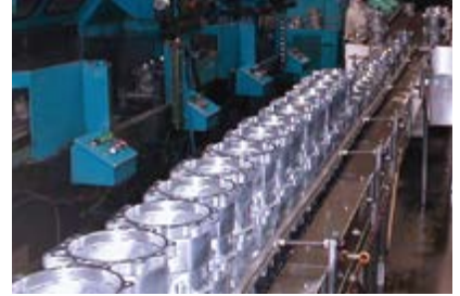
LOW LINE PRESSURE ACCUMULATION
